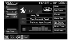
**Scan:** Press to hear a brief sampling of satellite radio channels within the currently selected genre. Press again to stop.
